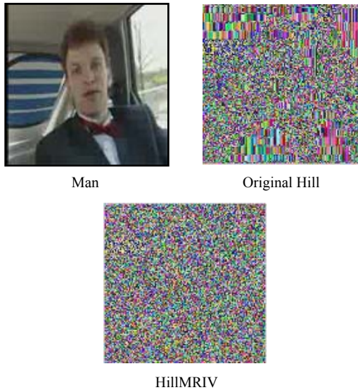
Fig.3 An example of color image encryption by the original Hill cipher and HillMRIV
